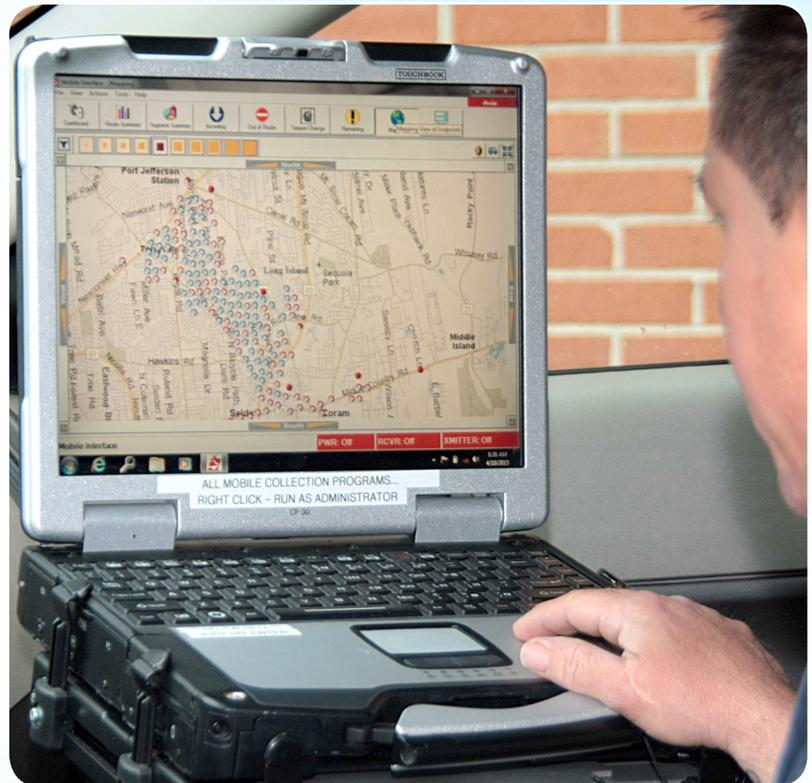
The use of AMR technology allows the Suffolk County Water Authority meter readers to collect reads just by driving past homes and businesses—a far more efficient process than reading meters manually. Here, a meter reader assesses progress in a neighborhood on a mobile computer.
