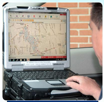
The use of AMR technology allows the Suffolk County Water Authority meter readers to collect reads just by driving past homes and businesses—a far more efficient process than reading meters manually. Here, a meter reader assesses progress in a neighborhood on a mobile computer.
